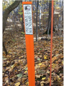
"Carsonite" boundary markers are placed at property corners where there is a survey pin.
